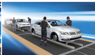
The Skid Transfer System
